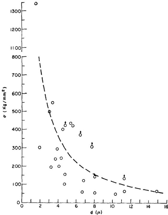
FIG. 6. The effect of size on the strength of iron whiskers.  $\delta$  fracture occurred at or near grips. True fracture stress may have been higher.
