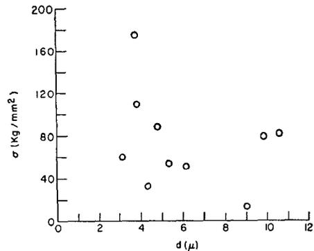
FIG. 8. The effect of size on the strength of silver whiskers.
